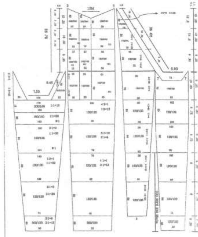
Figure 2: Drawing of the Custom Manufactured Bottom Trawl Net of the vessel.
